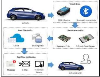
Fig. 4: Framework of Maintenance System
