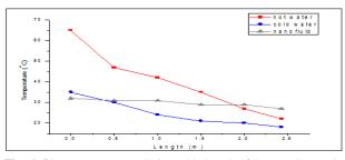
Fig. 6 (b): Temperature variation with length of heat exchanger in counter flow N-H-C arrangement using nano-fluid of 0.1% volume concentration
