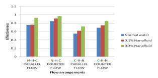
Fig. 7: Effectiveness of the heat exchanger at different flow arrangements
