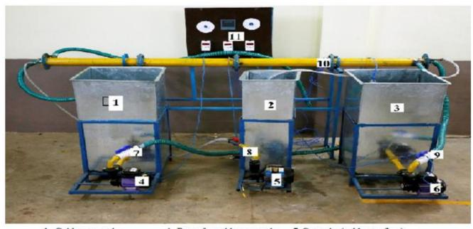
1- Cold water tank4- Pump for cold water tank7-Gatevalve(coldwater flow)2- Hot water tank5- Pump for hot water tank8- Gate valve (hot water flow)3- Nano fluid water tank6-Pump for normal water tank9- Gate valve (normal water flow)10- Test rig11- Data acquisition system
