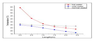
Fig. 6 (a): Temperature variation with length of heat exchanger in counter flow N-H-C arrangement using normal water
