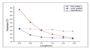
Fig. 6 (c): Temperature variation with length of heat exchanger in counter flow N-H-C arrangement using nano-fluid of 0.3% volume concentration
