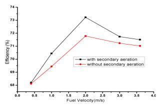
Fig.7: Comparison of thermal efficiency of the burner with and without secondary aeration.
