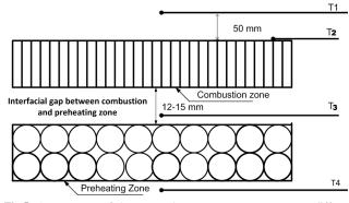
Fig.5: Arrangement of thermocouple to measure temperature at different locations of the burner
