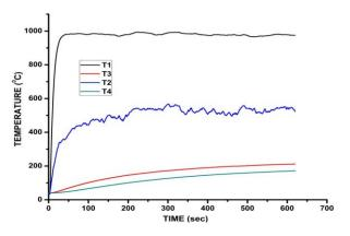
Fig6(b): Transient temperature distribution at different locations of the burner with secondary aeration
