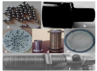
**Fig.3:** Components of the SAPSB (a) Stainless steel balls (b) burner body (c) perforated ceramic block (d) mixing tube with nuzzle (e) wire mesh with supporting frame (f) mixing tube with nuzzle and fuel ejector assembly.
