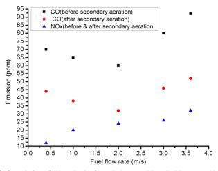
Fig.8: Emission of CO and NOx from the burner with and without secondary aeration
