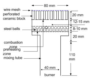
Fig.2: Schematic of the self-aspirated porous surface burner
