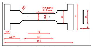
Fig. 6: Rectangular Cross-Section Tensile Test Specimen.
