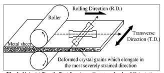
Fig. 1: Uniaxial Tensile Test Specimen Cut at an Angle of Orientation Relative to the Metal Sheet's Rolling Direction [16].
