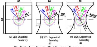
Fig. 9: Erichsen Cupping Test Specimen Geometries.
