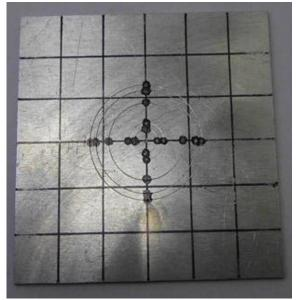
Fig. 8: Circle Grid Print on the Deep Drawing Test Specimens.
