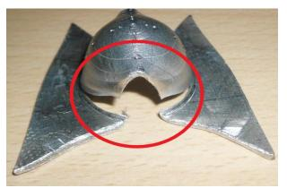
Fig. 17: Tearing, Excessive Thinning, and Earing.
