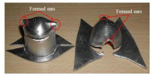
Fig. 18: Earing, Tearing, and Excessive Thinning.
