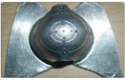
Fig. 13: Drawn Specimen (2.0 Mm) with Deformed Circles.
