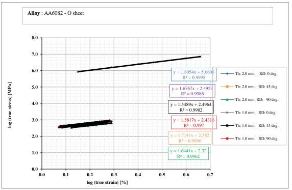
Fig. 12: Strain Hardening Exponent Determination by the Holloman-Ludwig Equation (Log  $\Sigma$  – Log E Plot).
