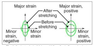
Fig. 4: Strain Analysis (Major and Minor Strain Determination).
