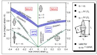
Fig. 5: Typical FLD Schematic by Keeler and Goodwin [14].
