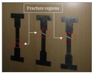
Fig. 10: Fractured Tensile-Test Specimens.
