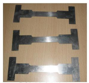
Fig. 7: Tensile Test Specimen Samples.
