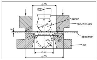
Fig. 3: Erichsen Cupping Test Principle [14].
