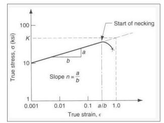
Fig. 2: Log True Stress-Log True Strain Curve [17].
