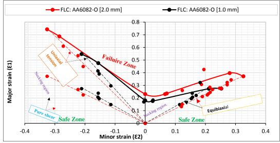
Fig. 19: Strain Measurements and FLD of AA6082-O Sheet Metal.
