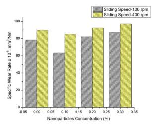
Figure 4: Nanoparticles concentration on specific wear rate.
