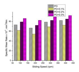
Figure 3: Effect of sliding speed on specific wear rate
