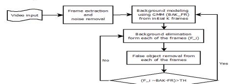
Figure 2: Work flow diagram of event detection
