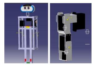
Figure 6. CATIA V5 model of the frame and arm [19]
