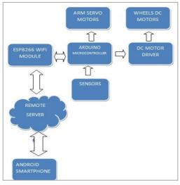
Figure 4. Block Diagram of Proposed Control System
