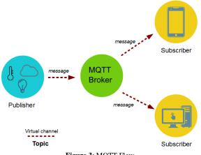
Figure 3: MQTT Flow
