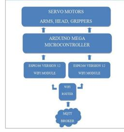
Figure 5. Servo Motor control
