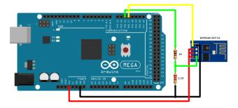
Figure 2: ESP8266 with Arduino Mega
