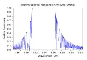
Figure 3. Reflected power vs wavelength
