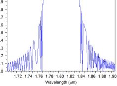
Figure 8. shows the graph of reflected power vs and wavelength for FBG4.
