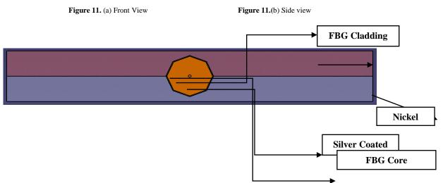
Figure 12. Metal FBG model discretization views in COMSOL Multiphysics
