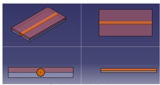
Figure 9. Metal Embedded FBG in different view
