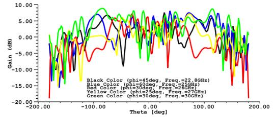
Fig.7. Gain of antenna for the frequencies (22 GHz-30 GHz).
