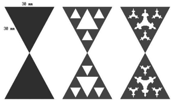
Fig.2. Antenna fractal shape: Second iteration of Seirpinski combined with modified Koch.
