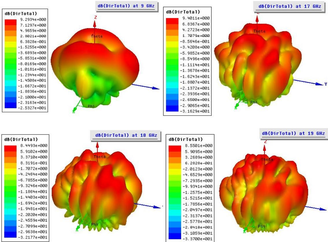
Fig.9. Three dimensional pattern of the antenna.
