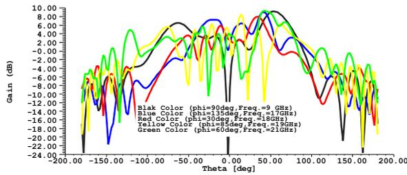
Fig.6. Gain of antenna for the frequencies (9 GHz-21 GHz)
