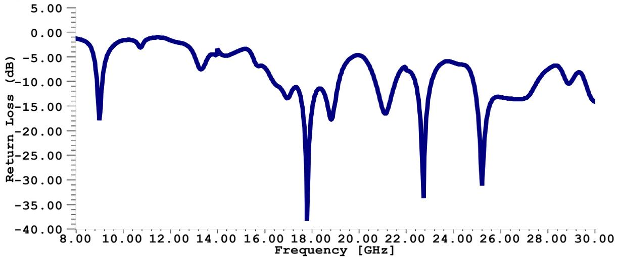
Fig.4. Return loss of the antenna.
