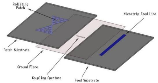
Fig.3. Feed configuration of the antenna.
