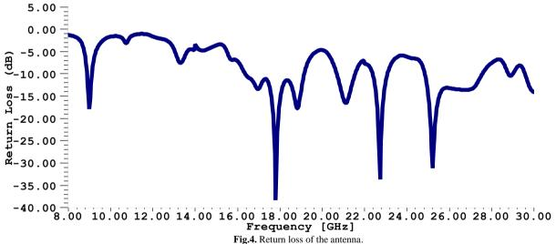
It is obvious from this figure, the principal frequency located at 9GHz and the other matching points located at frequencies of kband. This property of uniting too far apart bands in one single antenna makes it very useful in future wireless devices. The resistance of the feed line of the antenna is set to 50 ohm. Resistance versus frequency is shown in Fig.5.
