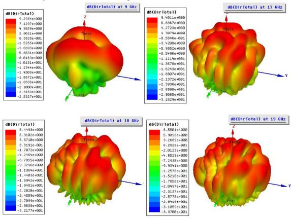
Fig.9. Three dimensional pattern of the antenna.
