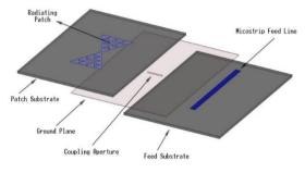
Fig.3. Feed configuration of the antenna.
