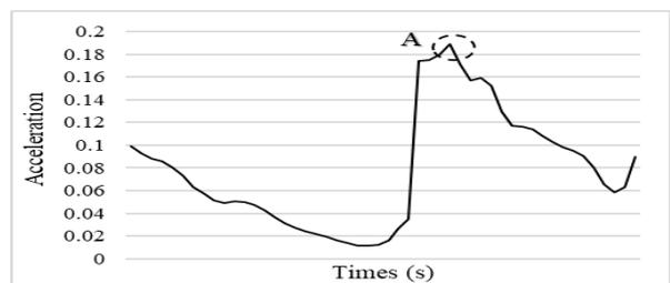
Fig. 8: Accelerometer Profile for a Drum Strike. Point A Indicated the Peak Acceleration when a User Touch on the Instrument Surface.
