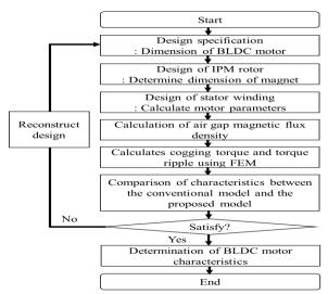
Figure 4: Proposed design algorithm of the BLDC motor for an EWP
