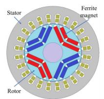
Figure 5: Proposed model of the IPM BLDC motor
