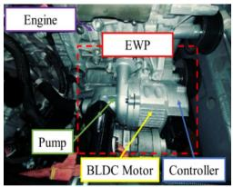
Figure 1: Structure of the EWP mounted on an engine
