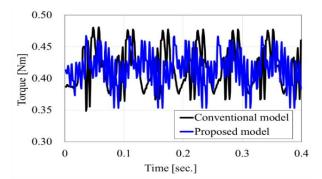
Figure 9: Comparison of the torque ripple characteristics (rated torque: 0.41 Nm)
