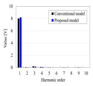
Figure 7: Comparison of the THD characteristics of the back-EMF
