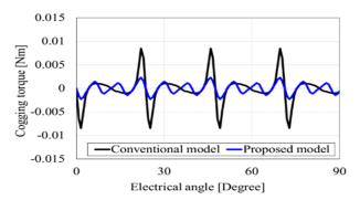
Figure 8: Comparison of the cogging torque characteristics (no-load condition)
