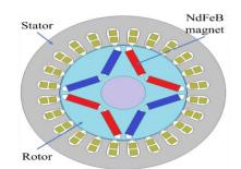
Figure 3: Cross section of an IPM BLDC motor (Conventional model)
