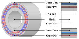
Figure 2: Structure of coaxial magnetic gear
