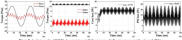
Figure 8: Analysis results of RCMG characteristics: (a) Pull-out torque, (b) Transient torque (c) Core loss (d) PM loss
