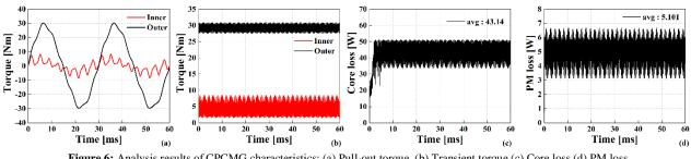
Figure 6: Analysis results of CPCMG characteristics: (a) Pull-out torque, (b) Transient torque (c) Core loss (d) PM loss
