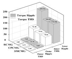
Figure 9: Three types of torque THD and torque ripple characteristics
