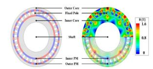
Figure 3: Structure and flux density and flux line of surface mounted coaxial magnetic gear
