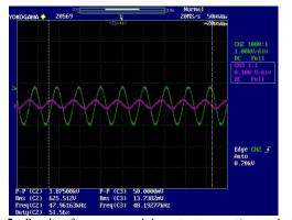
Figure 5: Result of power supply's output properties analysis by oscilloscope
