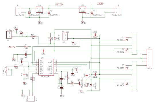
Figure 2: Circuit design of Power supply for small size low-pressure plasma surface treatment equipment
