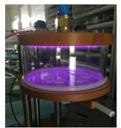
Figure 4: Low-pressure plasma surface treatment by developed equipment
