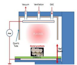
Figure 1: Diagrams of small size low-pressure plasma surface treatment equipment
