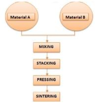
Fig. 3: Flow chart for Powder Metallurgy Process
