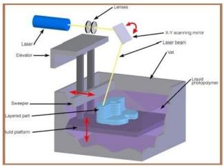
Fig.8: Stereo Lithography Process
