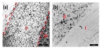
Fig.6: Microstructure of Al/ Al2O3 FG sample observed under optical microscope
