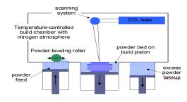
Fig. 9: Selective Laser Sintering Process
