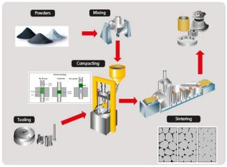
Fig. 4: Stages of Powder Metallurgy process
