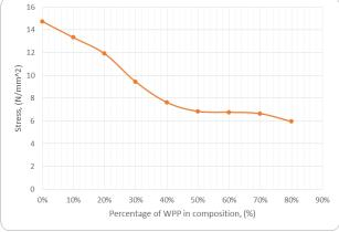
Fig. 5: Graph of stress versus WPC composition
