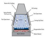
Fig. 2: UV accelerated weatherometer
