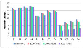
Fig. 5: Maximum strain of WPC samples before and after UV
