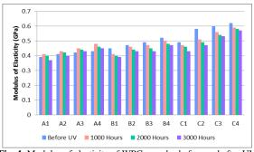
Fig. 4: Modulus of elasticity of WPC samples before and after UV
