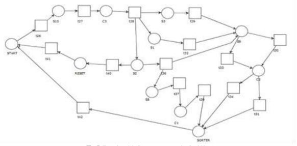
Fig. 7: Formal model of conveyor sorter using Petri Net
