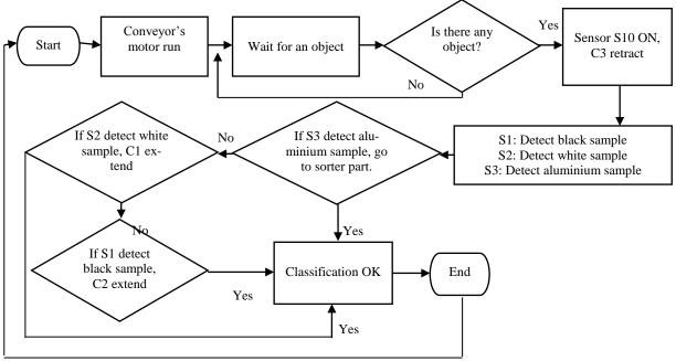
Fig. 4: Flowchart of conveyor sorter
