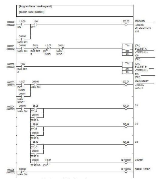
Fig. 5: A part of ladder diagram for conveyor sorter system
