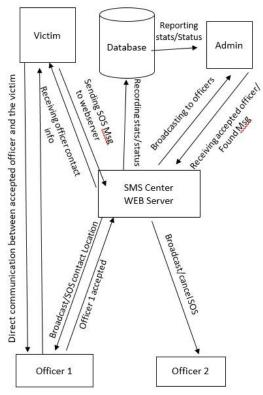
Fig. 2: Overall process when utilizing the SOS Banjir application
