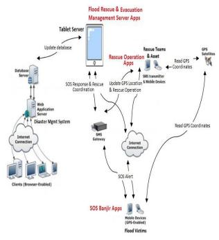
Fig. 1: The system architecture for the Flood Rescue & Evacuation Operation Management
