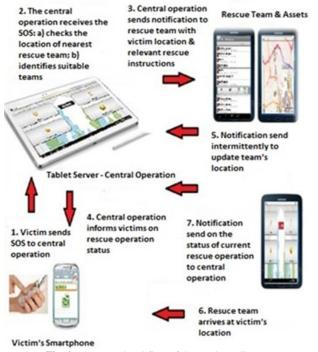
Fig. 4: The operational flow of the ResQ Banjir system
