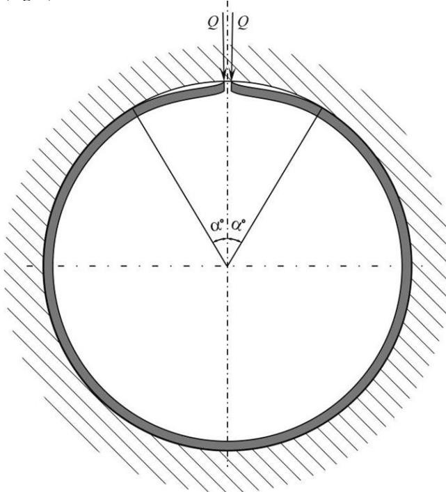
Fig. (2). Piston ring deformation model
