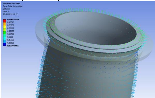
**Fig .( 4).** Temperature deformation of the upper part of the sleeve placed in the cylinder block.
