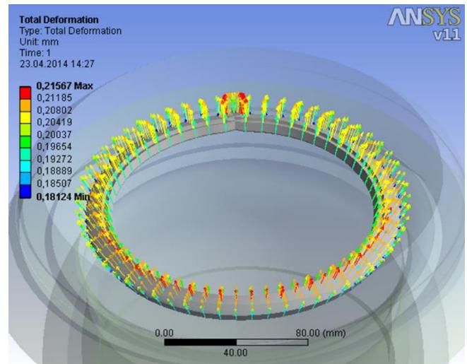
**Fig .( 5).** Deformations in an upper piston ring.
