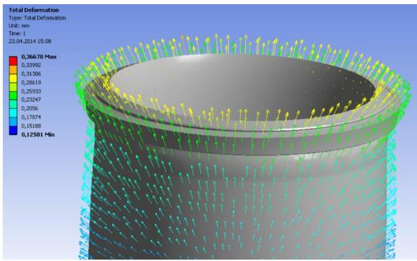
**Fig .( 3).** Temperature deformation of the upper part of the sleeve.
