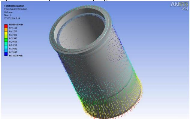
**Fig .( 5).** Deformations of rings and sleeves caused by temperature
