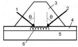
Figure 1. Diagram of the device with interference of evanescent near-field waves of a prism with full internal reflection based on [4]. 1, 2 — laser
