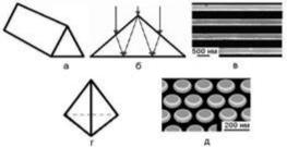
**Figure 5.** The use of laser interference lithography in the manufacture of 1D (ab) and 2D (d-e) magnetic meta-materials [10]: a is a glass prism, b is a beam path in a prism, c is a sample of 1D meta-material, d is a glass pyramid d - a sample of 2D material.
