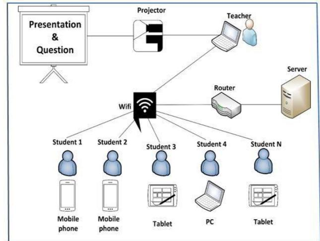
Fig. 1: Standard architecture of mobile-based CRS.
