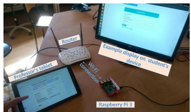
Fig. 5: The real implementation of the proposed architecture
