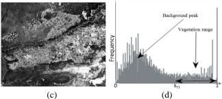
**Fig. 4:** Threshold based on histogram: (a) (c) Processed Hue and Saturation components, (b) (d) Histogram display of image data.
