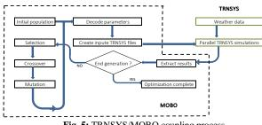
Fig. 5: TRNSYS/MOBO coupling process
