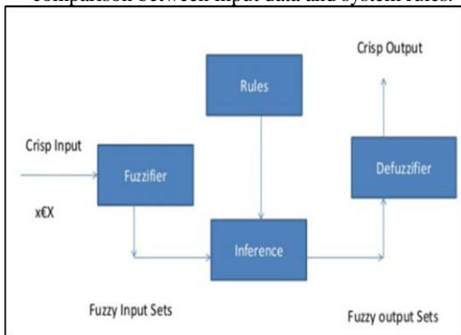
Fig. 6: System architecture
