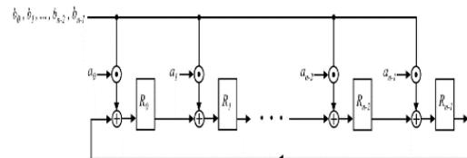
Fig. 1: Schematic of serial in parallel out multiplier
