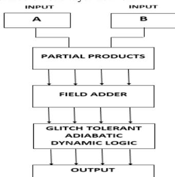
Fig. 2: Architecture of adiabatic logic design
