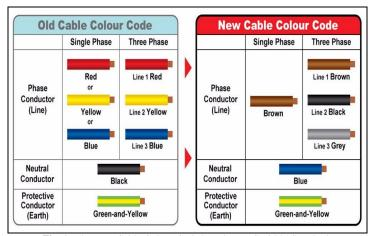
Fig. 1: The New Cable Colour Code based on IEC 60445 Standard.
