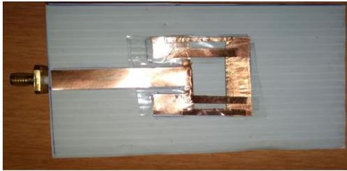
Fig.17: Fabricated softwear Antenna
