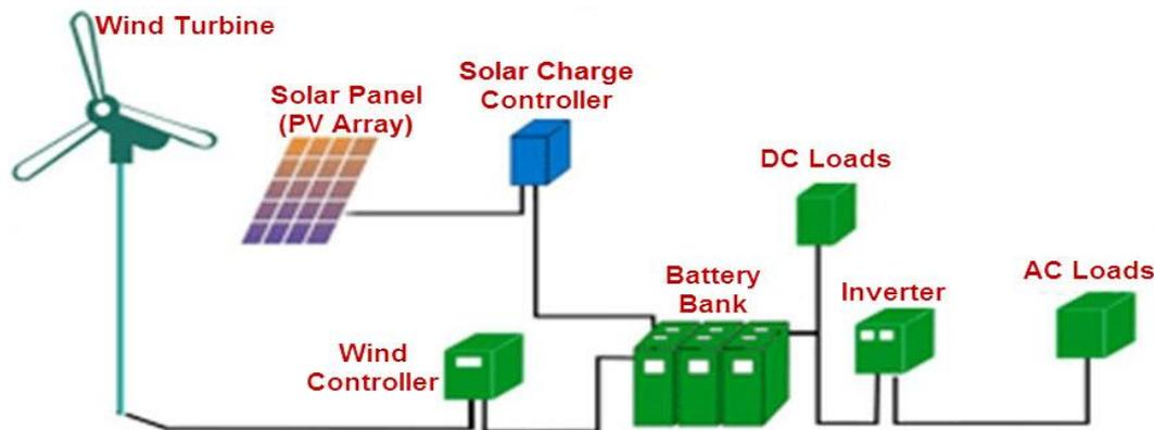
Figure.3: wind-solar system
