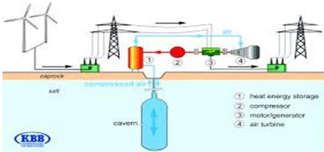
Figure.2 Wind-Compressed Air System
