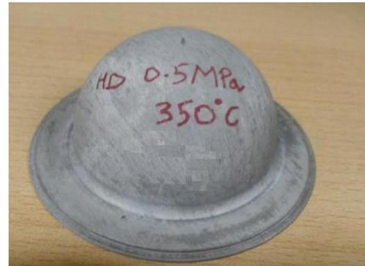
Figure 5: Specimen formed by superplasticity at 0.5 MPa, 350 °C of thickness 2.5 mm.
