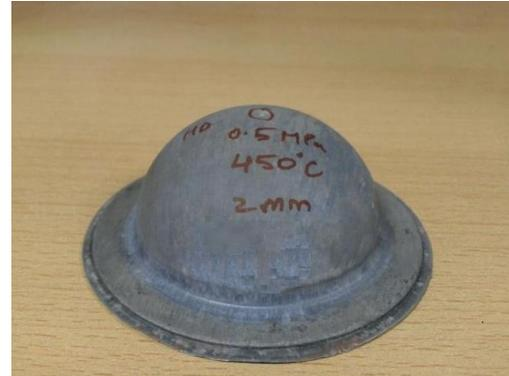
Figure 4: Specimen formed by superplasticity at 0.5MPa, 450 °C of thickness 2 mm.
