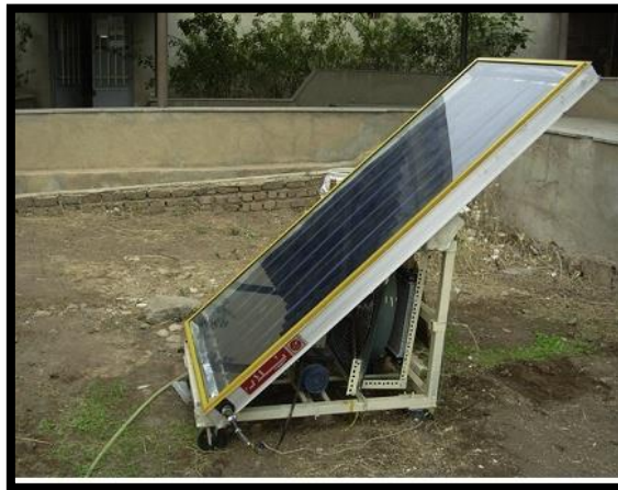
Fig 2.: Experimental work of solar collector using nanofluids [67].
