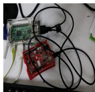
Fig. 7: Wired connection of Arduino and RPi
