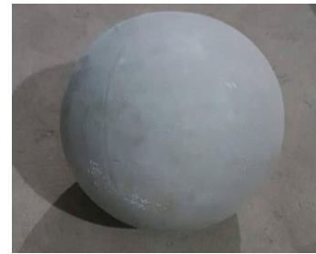
Fig. 2: Spherical shell made of fiber glass material
