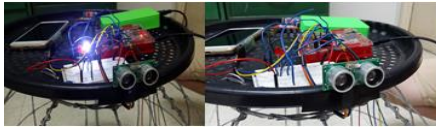
Fig. 6: Placement of ultrasonic sensors with obstacle detected (left) and no obstacle detected (right)
