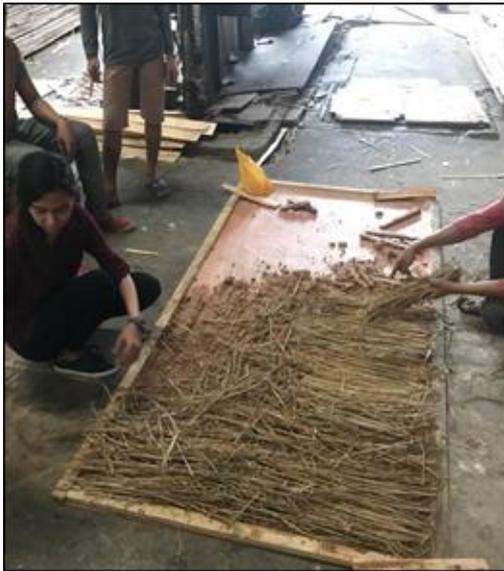
Fig. Placement of Rice Straws in the Mold : 4
