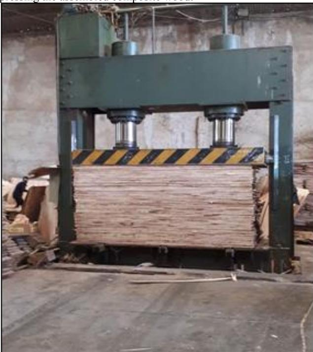
Fig. Cold Press Machine Pressing the Assembled Composite Wood : 5
