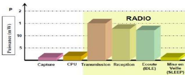
Fig.10. Energy consumption in a sensor node.
