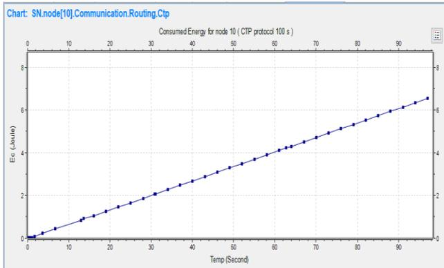
**Fig 15.** Consumed energy during 100s of simulation for CTP protocol.
