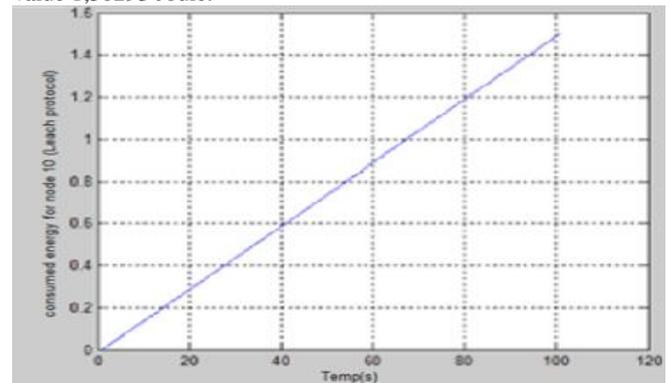
Fig.13. Consumed energy for node number 10 during 100s of simulation for LEACH protocol.
