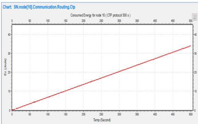
**Fig 16.** Energy Consumed during 500s of simulation for CTP protocol.
