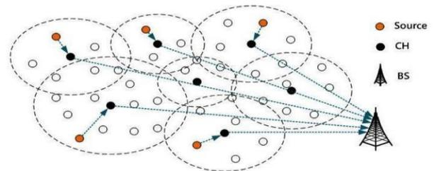
Fig 11. LEACH hierarchical routing architecture.
