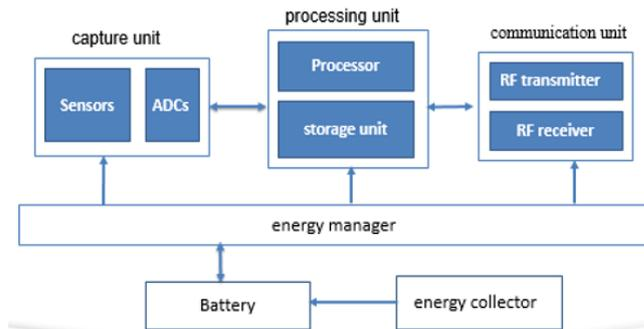
Fig 2. Sensor Node Architecture.
