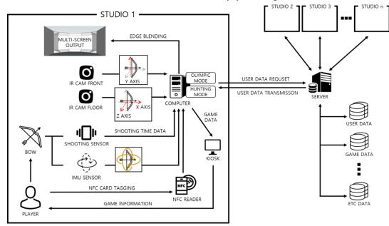
Figure 6: Structural diagram of the screen archery system using the VR shooter
