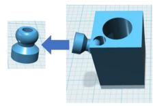
Figure 4: Example of case design to ensure flexibility between connecting lines
