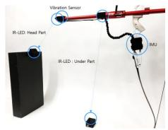
Figure 2: Structural diagram of the screen archery system using a VR shooter
