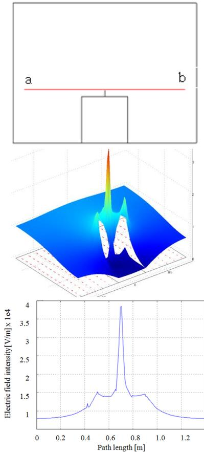
**Figure 2:** In case of ESE type, the electric field extraction path and field intensity
