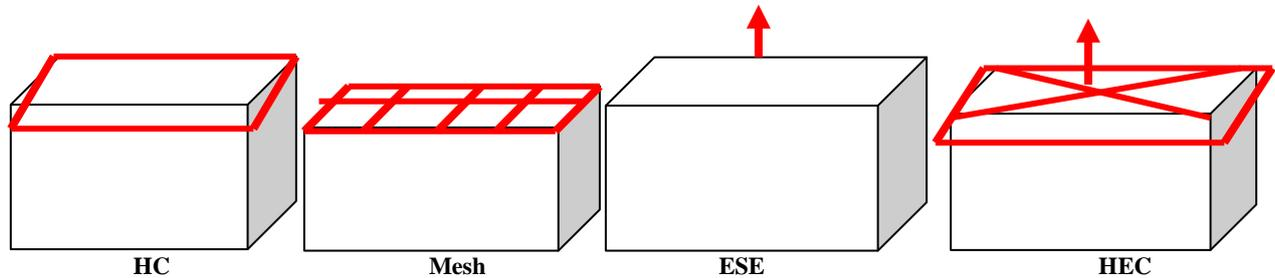
Figure 6: Various types of air termination for lightning
