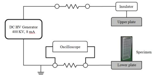
**Figure 4:** Installation map of high voltage generator
