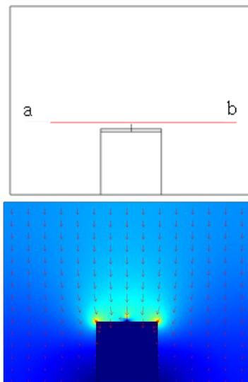
**Figure 3:** In case of HEC type, the electric field extraction path and field intensity
