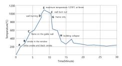
Figure 1: Fire process on wooden structure
