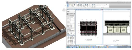
Figure3: BIM generation process in Bongjeongsa
