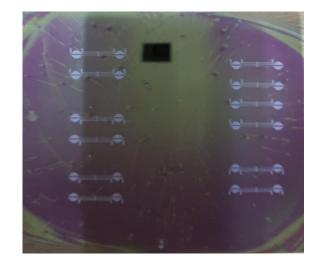
Figure2: Fabrication of ZnO thin film SAW filter by Photolithography
