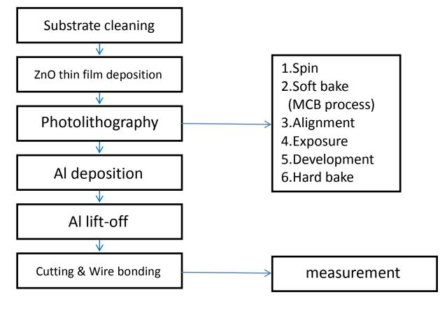
Figure 1: Fabrication process chart of ZnO thin film SAW filter
