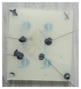
Figure3:.Cutting and wire bonding of ZnO thin film SAW filter
