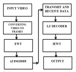
Fig 5: Video coding using wavelet and LZW coding
