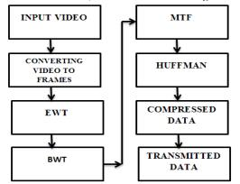
Fig 6: Video coding wavelet and combinations of BWT, MTF and Huffman coding
