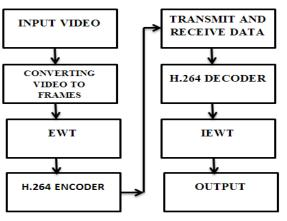
Fig 1: Video compression using EWT and H.264
