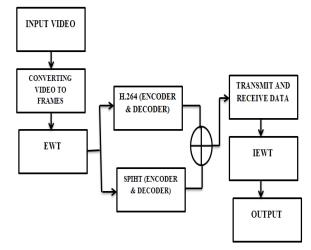
Fig 3: Video coding using wavelet and combination of H.264 and SPIHT
