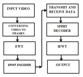
Fig 2: Video coding using wavelet and SPIHT
