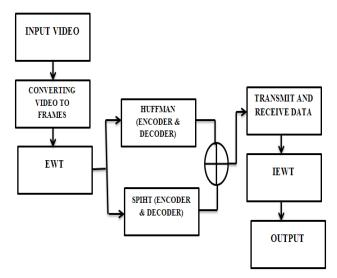
Fig 4: Video coding using wavelet and combination of Huffman and SPIHT.
