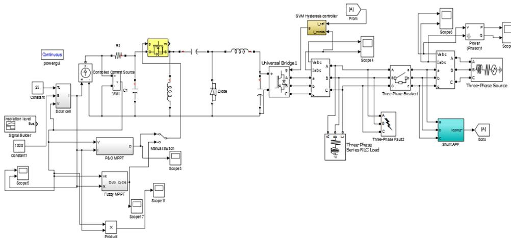
Fig. 6.:Proposed PV system using MATLAB/SIMULINK
