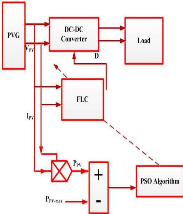
Fig. 1: Standalone PV controlled using PSO-FLC
