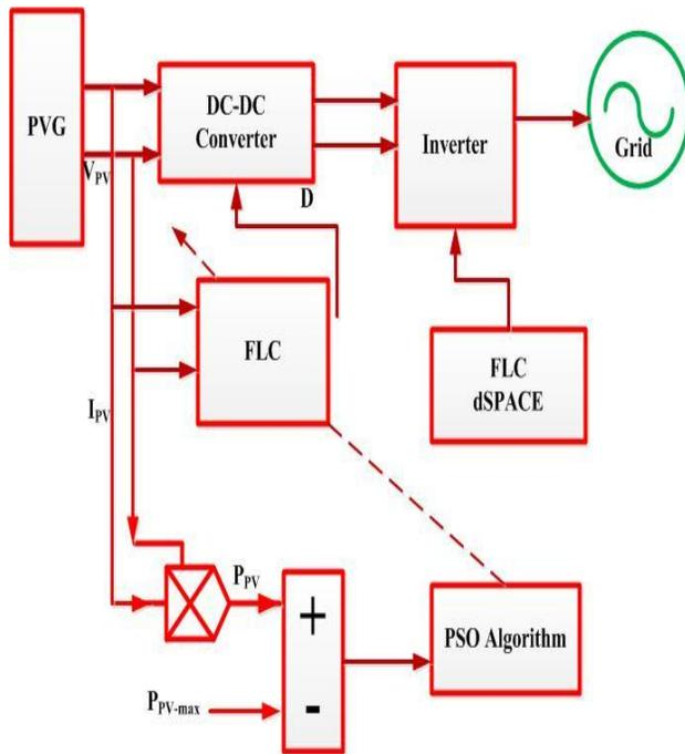
Fig. 2: Grid connected PV controlled through PSO-FLC
