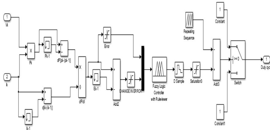
**Fig. 4.:** Fuzzy based MPPT controller designed using MATLAB
