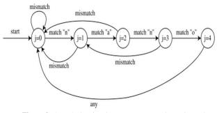
Figure 3: A DFA showing the pattern text match or mismatch
