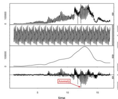
**Figure 1:** An example of the STL technique with original time series, seasonal, trend and residue parts graphically represented from top to bottom.
