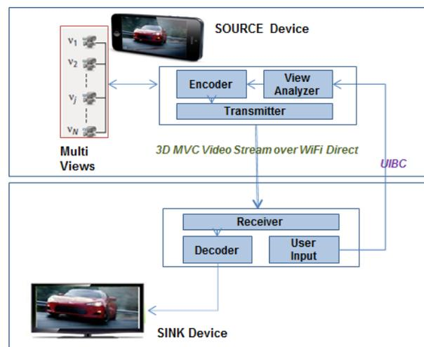
Fig. 4: System Architecture
