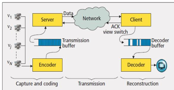
Fig. 3: Multi-view video delivery system architecture
