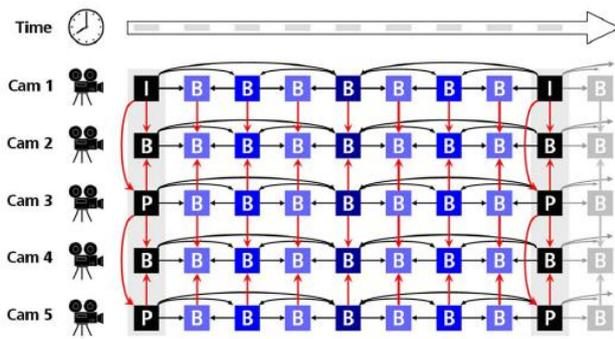
Fig. 2: MVC Prediction Structure with N=5
