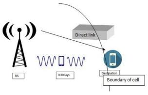
Figure 1: Illustration of a co-operative system.
