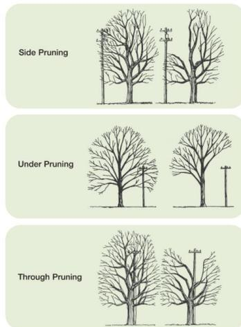
Fig. 1: Pruning method being used by Nasional Grid
