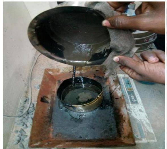
Fig 3.1: Preparation Of Blends (Pvc+Bitumen)
