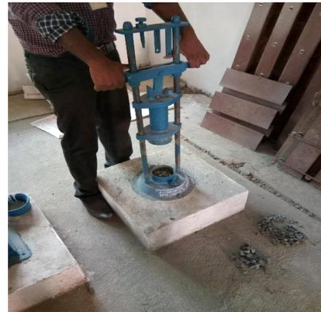
Fig 3.3: impact test
