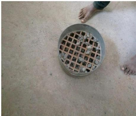
Fig. 3.2: gradation of aggregates
