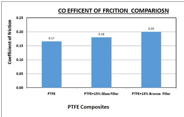
Fig 7: Coefficient of friction of PTFE and PTFE composite
