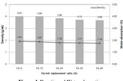
Figure 4. Density and Water absorption
