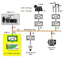
Figure 1: Configuration of Geocha island MG
