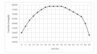
Figure 4: Total Energy Obtain Ratio until Replacement Time of Li-ion Battery
