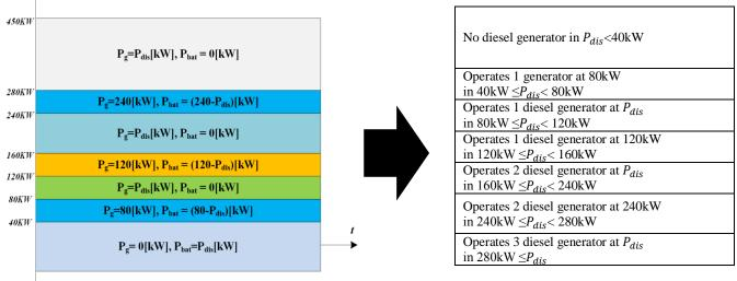
Figure 5: Design of Optimal Operation Algorithm for MG
