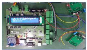
Figure 9:. Main control board of LED security light
