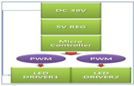
Figure 1: LED Driver PWM Control Block Diagram
