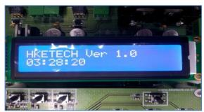
Figure 10: Initial output screen of LCD(Display present time)
