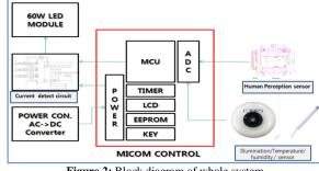
Figure 2: Block diagram of whole system
