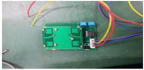
Figure 5: RF sensor detecting motion of human body and thing
